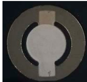
Figure 9: Freestanding, thermally and mechanically decoupled resonator
