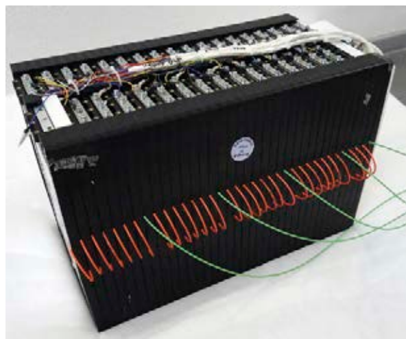
Figure 2: Battery block with fibres
