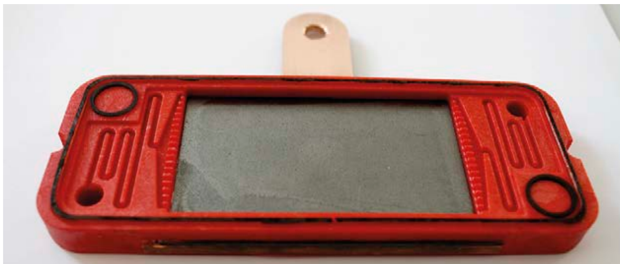
Figure 2: Injection-moulded frame with cast-on monopolar plate and current collector.
